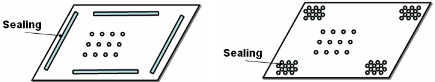
Figure 8. Sealing layout as additional strength for three-dimensional chip stack.
