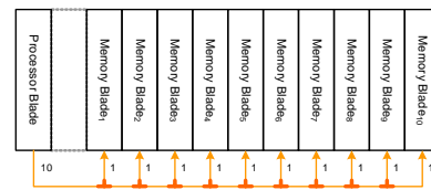
Figure 4: Optical Backplane Example with 11 Blades Variable splitting ratio = 1:9, 1:8, 1:7, \dots, 1:1
