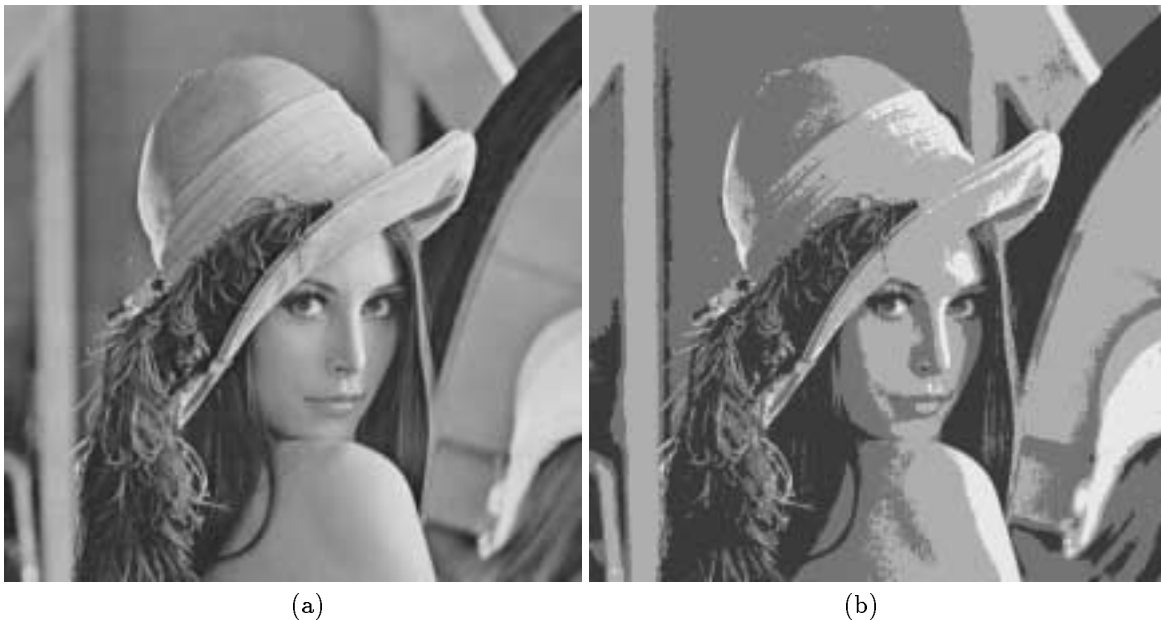
Figure 4. (a) Lena image. (b) Lena image after quantization with step 58. Posterization and contouring appear due to the quantization.
