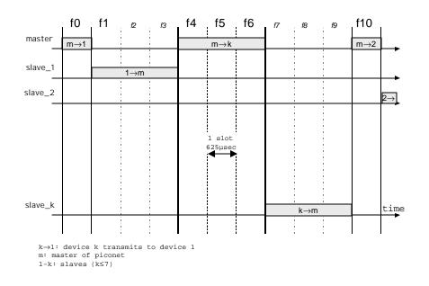
Figure 2: Transmissions in a Bluetooth piconet
