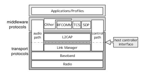
Figure 1: The Bluetooth protocol stack
