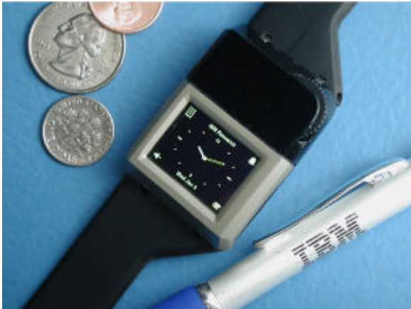
Photo 1 OLED display in a computer wrist watch
