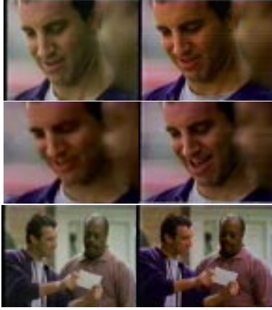
Figure 1: Images taken from different sources. Top-left: 176 \times 112 MPEG1. Top-right: 160 \times 120 AVI. Middle-left: RealVideo 28k ( 160 \times 120 ). Middle-right: RealVideo 512k ( 160 \times 120 ). Bottom-Left: MPEG1. Bottom-Right: AVI
