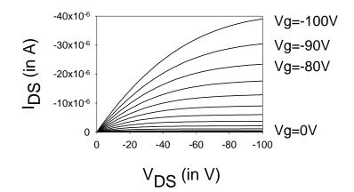
Fig. 2. Current-voltage characteristic of an OTFT produced using this process. The performance observed is what we had measured from shadow-masked, bottom-contact OTFTs. Channel width, W=1500  $\mu$ m, channel length, L=70  $\mu$ m
