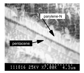
Fig. 3. A micrograph of a field effect transistor etched using this process. The edges of pentacene and parylene are clearly visible.
