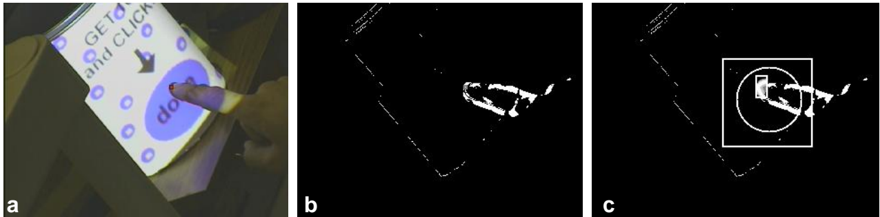
Fig. 3. a) Camera view of an interaction with a bucket; b) image difference data; c) overlay of search region (square), button active area (circle), and the fingertip template shown at the pointing location.
