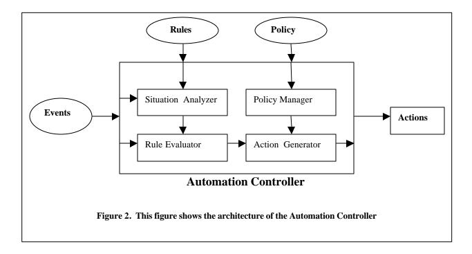
In the AC, each system management task is represented as a set of rules that specify the behavior of the system for a particular request. The requests are received as events. The situation analyzer correlates the incoming events and tries to determine the situation. The information is then passed onto the rule evaluator. As the situation analyzer is responsible for determining the problem situation, it acts like a "sensor" of an agent.
