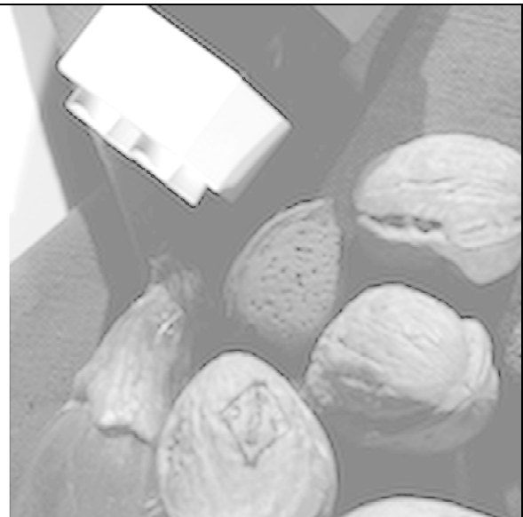
Figure 4b. A section of Figure 3a after severe low-pass filtering enlarged to show loss of high frequency detail.
