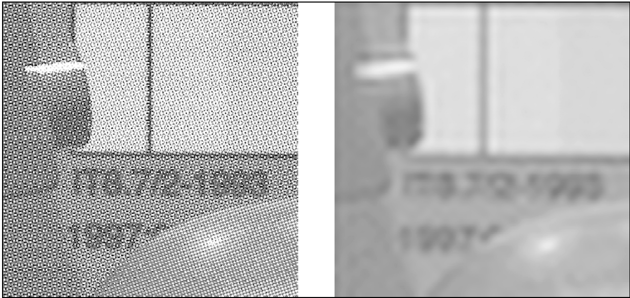
Figure 5a. A section of Figure 3a enlarged to show high-energy high-frequency artifacts caused by halftoning .
