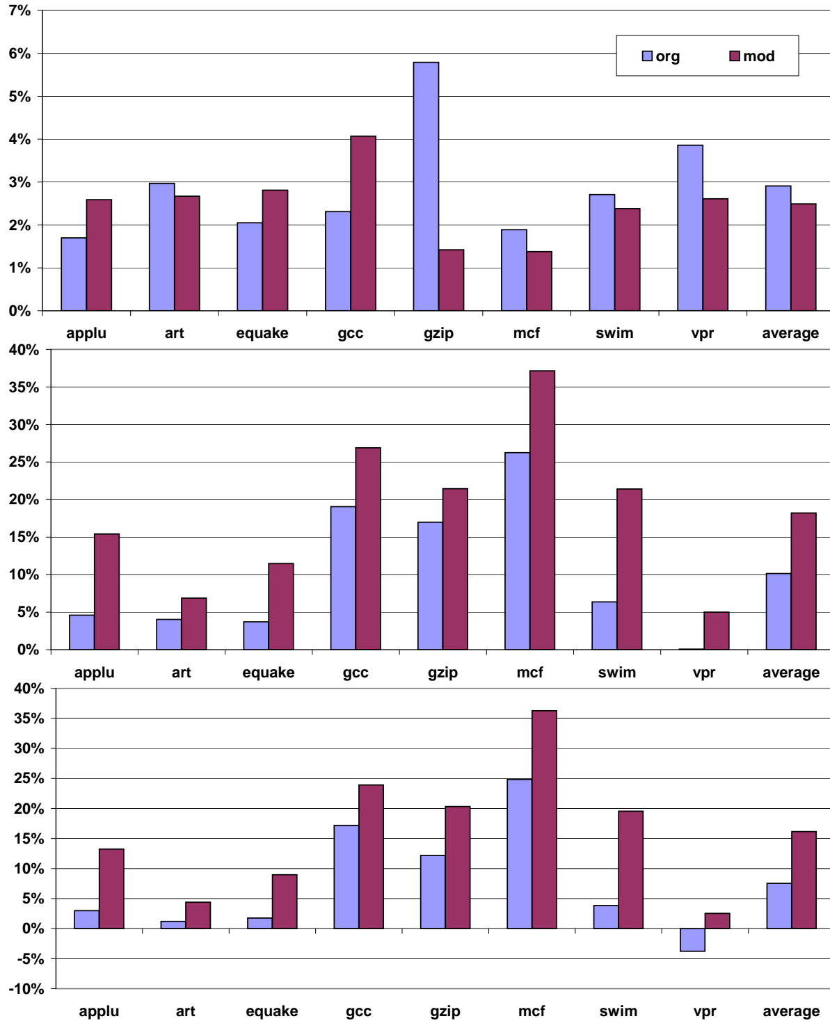
Figure 11. Performance degradation (upper), energy savings (middle) and energy x delay improvement (bottom), over a fully synchronous machine with the same architectural parameters. org stands for the original MCD design with the original online algorithm using full-frequency scheme; mod stands for the new domain partition scheme with our modified online algorithm and four frequencies/voltages.
