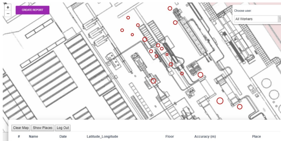
Fig. 5. Live map from indoor location platform (large factory pilot)
