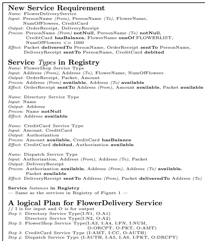
Figure 3: The proposed modeling for FlowerDelivery scenario with service types, roles and NFRs.
