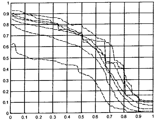
Figure 4. Retrieval precision-recall for speech recognition alone, as it changes according to the query word length in phones from three (bottom curve) to 15 (upper curve).
