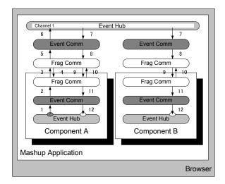
Figure 3. Layered component communication
