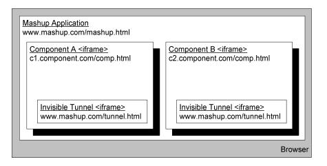
Figure 2. Fragment communication architecture
