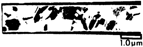
Fig. 1. Focused ion beam micrograph showing the grain structure of the CVD Cu lines.
