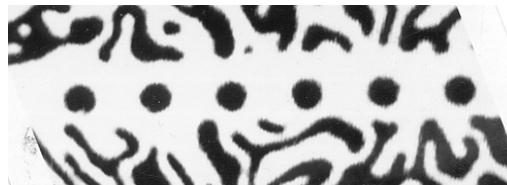
Fig. 12. Pure polar Kerr-effect contrast in a magneto-optic media film (method of Fig. 11 adapted from [17])
