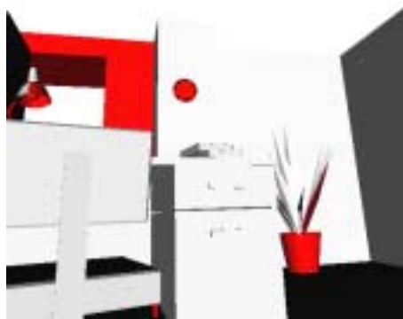
Figure 2: Illustration of the accuracy of PLP: For the same viewpoint and model as shown in Fig. 1, the visible geometry that PLP rendered is shown in white, and the visible geometry that PLP did not render is shown in red.
