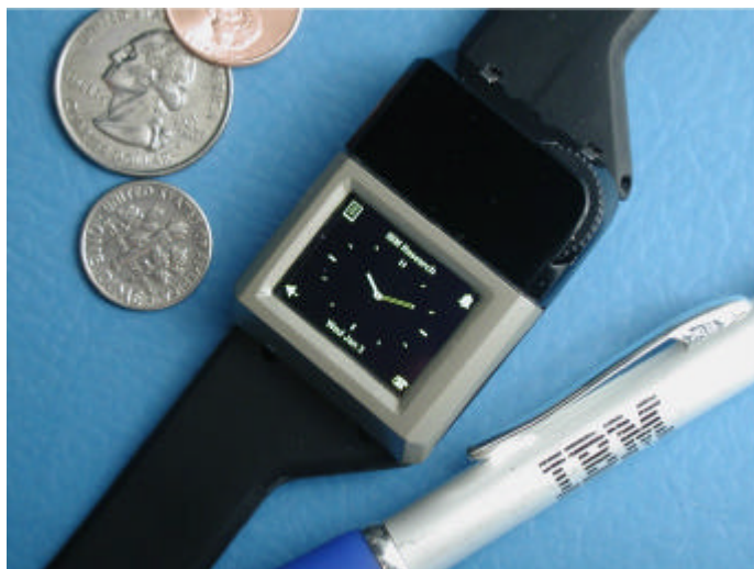
Photograph 1: The OLED VGA on crystalline silicon display is shown in a Linux computer wristwatch prototype.
