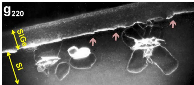
Fig. 3: Cross-sectional TEM micrograph (weak beam conditions) showing platelets below the Si/Si 1-x Ge x interface in sample 2 of group 2. From these platelets, dislocation loops extend in all 8 <110> directions and glide to form misfit dislocation segments at the interface as indicated by arrows.
