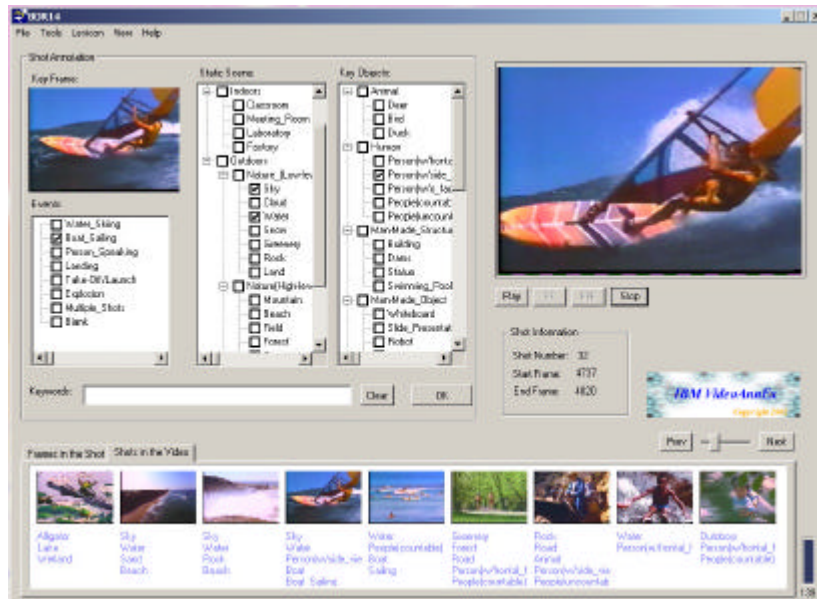
Figure 3: The IBM VideoAnnEx MPEG-7 Video Annotation Tool is divided into Four Regions: (1) Video Playback, (2) Shot Annotation, (3) Views Panel, and (4) Region Annotation (not shown).
