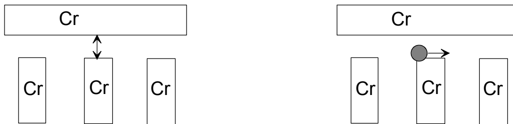
Figure 11: (a) The gap between 2 Cr features is measured using the DUV image available in the repair tool. A thin slice of Cr is ablated (b) and the gap is remeasured. DUV images of the Cr pattern illustrating the process is shown in Figure 12. The process is repeated many times to obtain the data shown in Figure 13.
