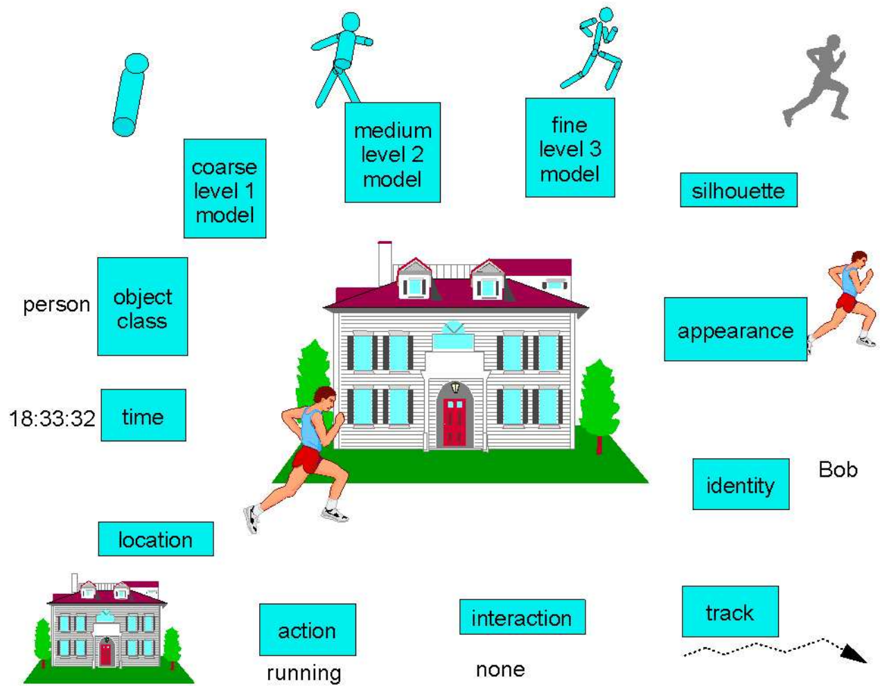
Figure 3: Video re-rendering options. The central image shows a video frame. Surrounding it are different methods of re-rendering the video which can be selected or composed together if the operator's privileges allow.
