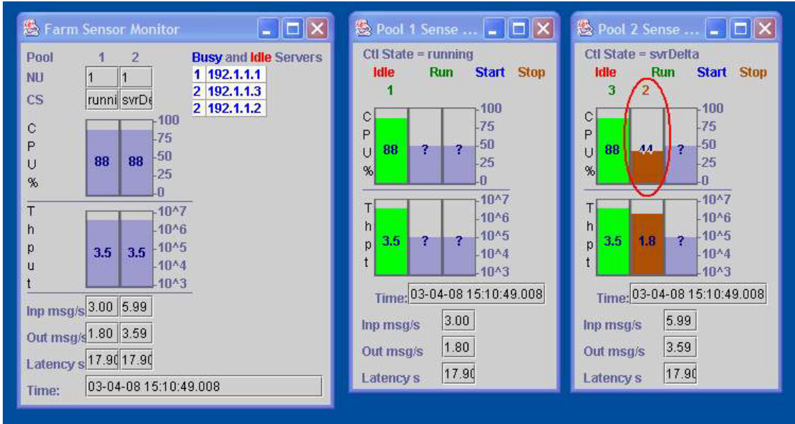
Figure 10 – Removing Server 2 from Pool 2
