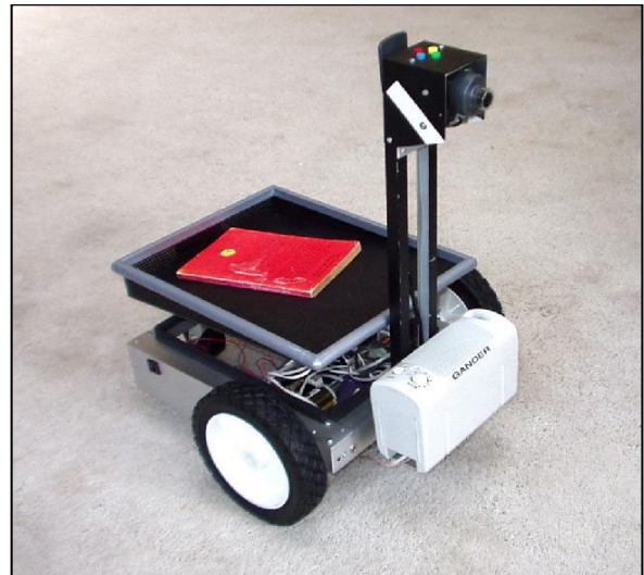
Figure 1. Our robot, “Gander”, has a dual-wheel differential drive and a wide-angle video camera. It is designed to carry items in a basket on its back.
