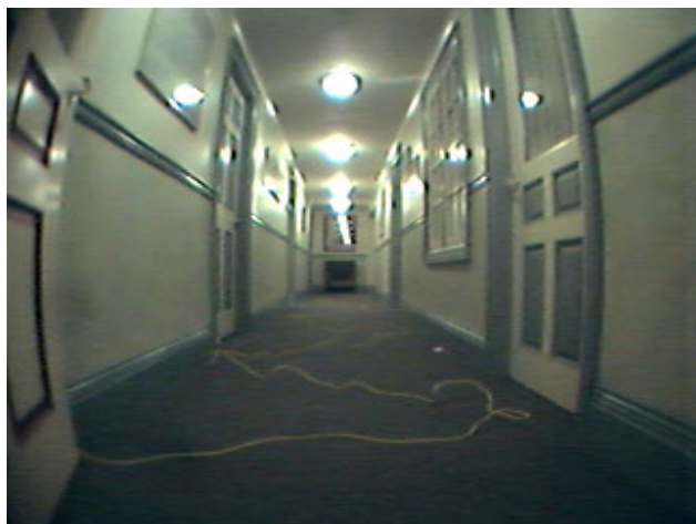
Figure 6. This is the hallway that was used in the experiments. The "torture track" was made by zig-zagging a 1/4 inch nylon rope diagonally across the hallway. This would defeat most wheel turn-counting odometry systems.
