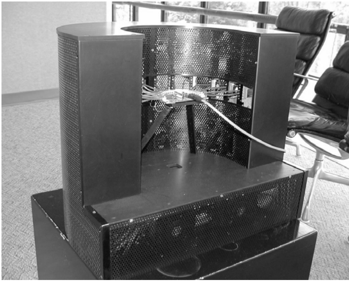
Fig. 8 Photograph of the custom 120 Gb/s testing tower. The optical transmitter is visible in the center and has a 12 fiber ribbon attached.
