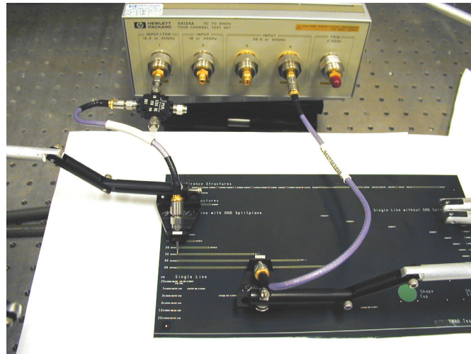
Fig. 10 Test measurement set-up showing the differentiator in-line with the sampling oscilloscope step source and the coaxial probes using for probing the various lengths lines.
