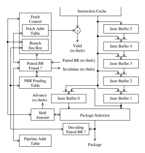
Figure 3 - Decoupled fetch-execute architecture with static branch prediction support
