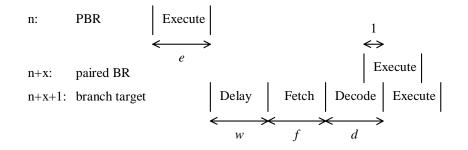
Figure 2 – Minimum latency between a PBR operation and its paired branch is x = e + w + f + d - 1 cycles
