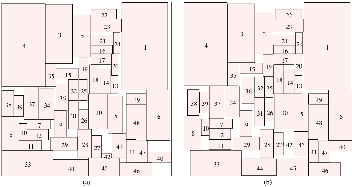
Figure 10: (a) The original ami49 placement in FAST-SP. (b) The new placement result when minimizing wire length in the same frame.
