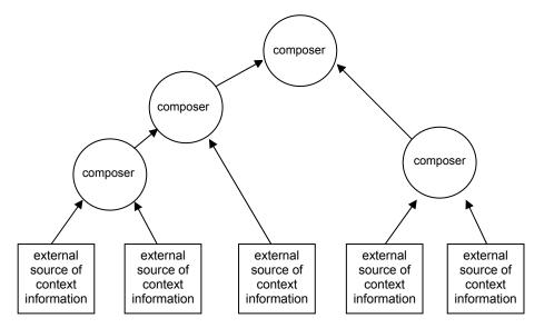
Figure 1. A tree of data providers. The leaves of the tree are external data sources and all other nodes of the tree are composers.
