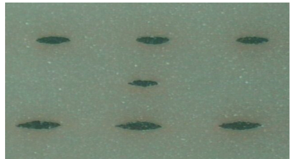
Fig. 8 Cross section of single-line site on layer six with mesh ground planes on layer five and seven.
