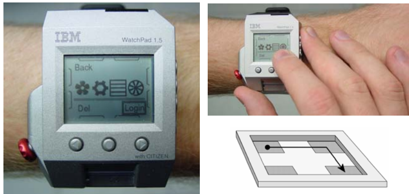
Fig. 5. (left) IBM/Citizen WatchPad, displaying pictogram-based authentication challenge interface. (right) User can locate tangible corner features of the WatchPad without looking at the device and may execute gestures by dragging the finger along the display's frame, using corner features as starting and stopping landmarks.
