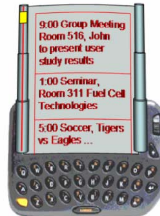
Figure 5: Display partially unrolled
