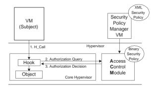
Figure 4: Hypervisor-based security reference monitor.
