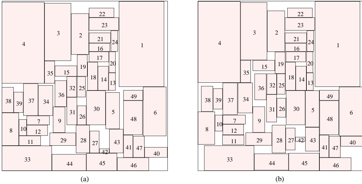
Figure 10: (a) The original ami49 placement in FAST-SP. (b) The new placement result when minimizing wire length in the same frame.
