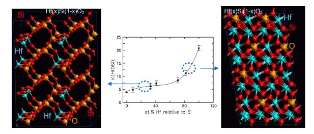
Fig. 2. Hf silicate structures which may form after a high temperature annealing of  $W/HfO_2/SiO_2$ . Center is a plot of silicate dielectric constant as a function of Hf at. % relative to Si<sup>11</sup>. At low Hf content the silicate structure is a SiO2 matrix with Hf embedded (left). At high Hf content the silicate structure is a HfO<sub>2</sub> matrix with Si embedded (right).
