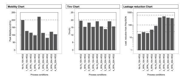
Fig. 5. Electron mobility, inversion layer thickness and leakage reduction charts of a W(= $20\mu$ m) x L(= $5\mu$ m) N-FET as a function of various RF nitridation processes of interfacial layer only. The gate stack was annealed at 1000 °C. Data are shown for two different HfO<sub>2</sub> thicknesses, 1.5 and 2.5 nm.
