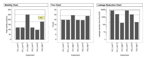
Fig. 3. Electron mobility, inversion layer thickness and leakage reduction charts of a W(= $20\mu$ m) x L(= $5\mu$ m) N-FET as a function of annealing temperature; LowT1~500 °C, High T~1000 °C. Gate stack is W/HfO<sub>2</sub>/SiON. In Ex2 the SiON layer was spike annealed at 1100 °C, in Ex1 the SiON was not spike annealed.
