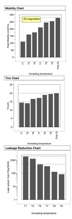
Fig. 1. Electron mobility, inversion layer thickness and leakage reduction charts of a W(= $20\mu m$ ) x L(= $5\mu m$ ) N-FET as a function of annealing temperature; T1~400 °C, T9~1000 °C. Gate stack is W/HfO<sub>2</sub>/SiO<sub>2</sub>.
