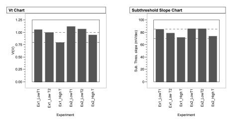
Fig. 4. Threshold voltage and sub-threshold slopes charts of a W(=20 $\mu$ m) x L(=5 $\mu$ m) N-FET as a function of annealing temperature; LowT1~500 °C, High T~1000 °C. Gate stack is W/HfO<sub>2</sub>/SiON. In Ex2 the SiON layer was spike annealed at 1100 °C, in Ex1 the SiON was not spike annealed.
