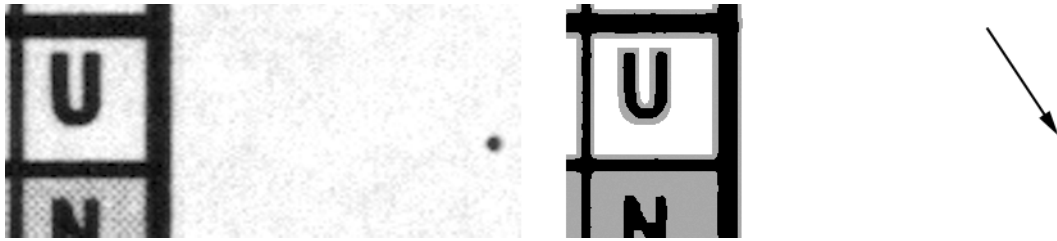
Figure 7: Scanned Image (left) showing defect in the paper, with Detection Image (right) showing detection of the defect (arrow) as “unexpected-black.”
