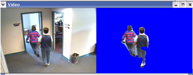
Figure 2 Output of the Background Subtraction (BGS) system.
