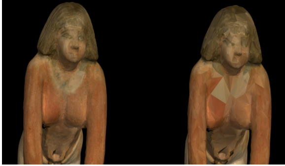
Figure 4. Drawback of 3D paint programs that require simplification: severe artifacts appear when the texture is re-mapped onto the simplified model.
