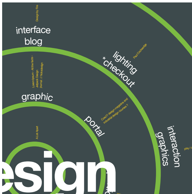
Figure 5. Close up of a TagOrbital for the “design” tag, showing some tags for band one (“graphic” and “portal”) and tags pairs for band two (“interface, blog”, “lighting, *checkout”, and “interaction, graphics”). The small radial lines of text are bookmark titles. Small clusters of these titles (which use the same tag) can be seen for the “graphic” and “portal tags.
