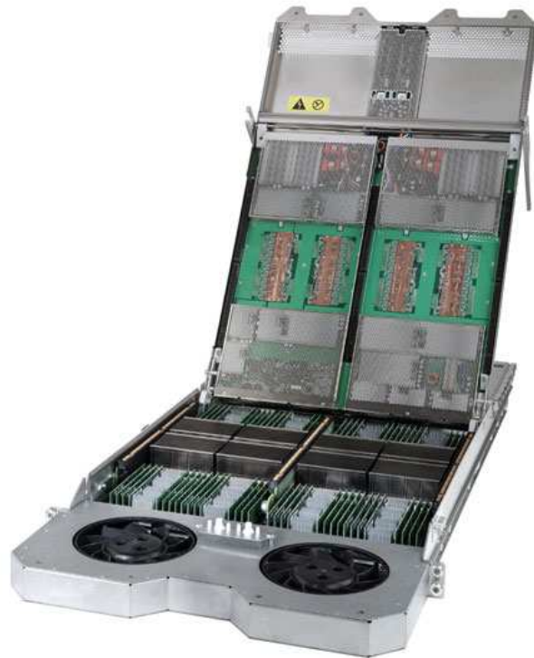
Figure 1: The POWER5 p5 575 SMP server.
