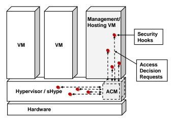
Figure 2: sHype Access Control Architecture
