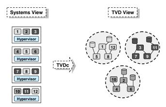
Figure 1: Trusted Virtual Domain View
