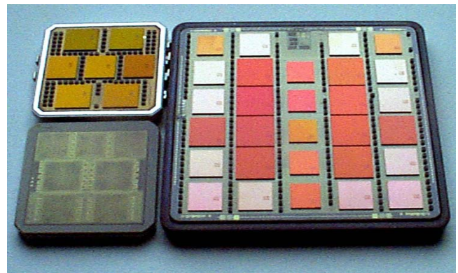
Figure 4: Modules built with discrete spacer [35]
