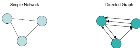
Figure 1: A simple network is defined by nodes and connections (one or zero per node pair), whereas the graphs simulated by the Simulator consist of vertices joined by any number of directed edges.
