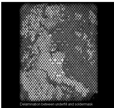
Figure 12. Delamination between underfill and solder mask found with CSAM. Delamination can be caused by underfill cure problems and surface contamination
