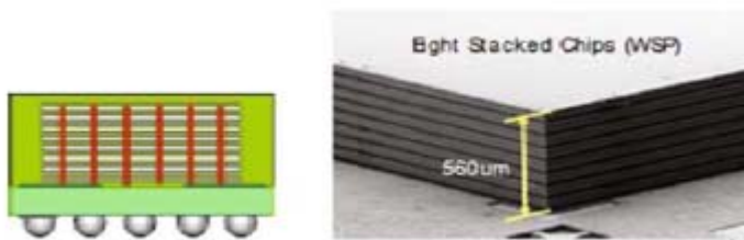
Figure 58. Samsung's 16 Gb memory module made with an 8-die stack using Cu-Sn-Cu technology [136].
