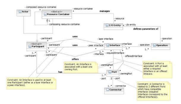
The elements in the figure above represent all the models and their relationships. However, in an actual engineering system, it is not necessary to exploit every model element and all its relationships.
