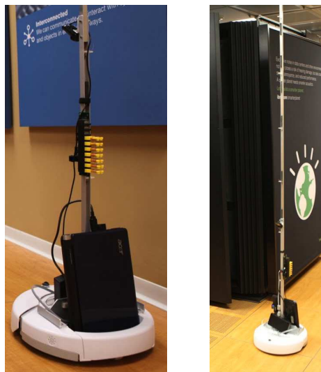
Fig. 1. The THOMAS system developed for data center monitoring
