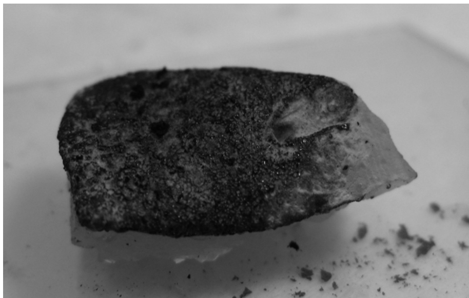
Figure 2. Pig skin sample, measuring \sim 2 \text{ cm}^2 in area, after exposure to the flame of a propane torch. The burn eschar is clearly seen on the surface of the skin.
