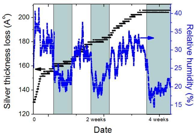
Fig 3 Silver thickness loss and simultaneous variation of the relative humidity in the data center. When the relative humidity goes below 27% (shaded regions) the metal loss became constant.
