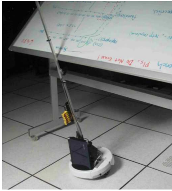
Figure 5: The robot getting upended in a futile attempt to scoot under a mobile whiteboard left in the data center.
