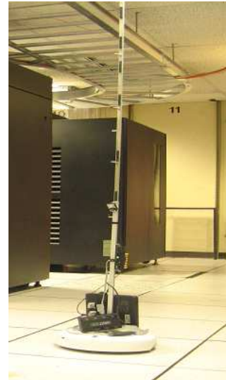
Figure 1: The data center management robot. generated layout as reflecting the physical layout of the data center.
